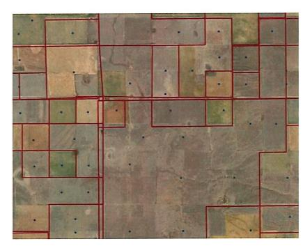
Figure 7: Rural areas also have issues with gaps and overlapping line work.
