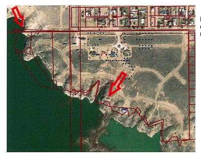
Figure 2: The line work has considerable gaps/overlaps in multiple locations.
