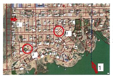
Figure 1: (1) UPC points appear to be incorrectly placed. This could not be corrected with a spatial adjustment. (2) Curve construction appears to be incorrect. (3) Line work for the area is shifted approximately 140' west of where it should be in this location.
