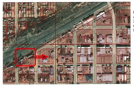
Figure 6: All blocks in this area appear to be shifted 300' west and slightly south of where they should be.
