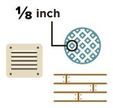
Install 1/8-inch metal mesh screens over vents and under decks to prevent ember intrusion.
